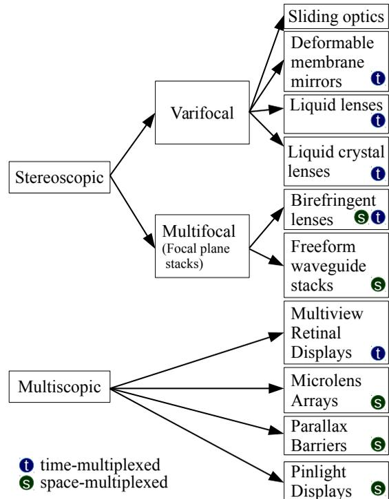
Figure 2. Classification tree of various display designs relevant to HMDs that have shown potential in resolving VAC.
