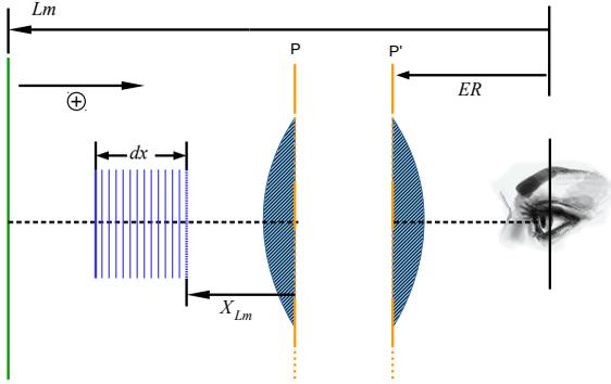
Figure 5. Basic layout of a magnifier as adapted from Rolland et. al in [48].  $Lm$  corresponds to  $d_{ei}$  in our nomenclature,  $X_{Lm}$  is  $d_{sl}$ ,  $ER$  is  $d_{el}$ , and  $dx$ , the stack thickness, is  $t$ . Note that the  $x$  axis is inverted relative to direction of these vectors.
