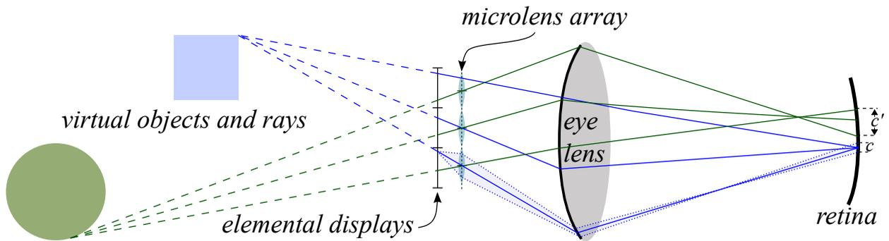
Figure 4. Conceptual diagram of a microlens head-mounted display. Eye is focused on the corner of the virtual blue box, while the green sphere appears out-of-focus.
